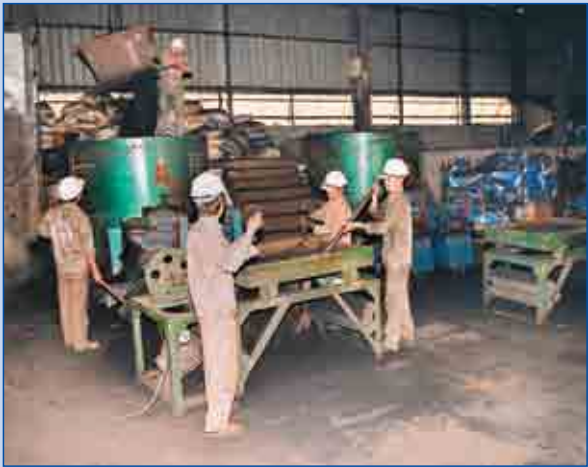
Making Moulds by Sand Technique
